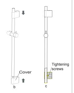
a).Be noted to keep top and bottom holders in alignment and same distance; then push assembled top & bottom cover with rail bar to the holders,and ensure the locking hook is locked into the locking slot.
