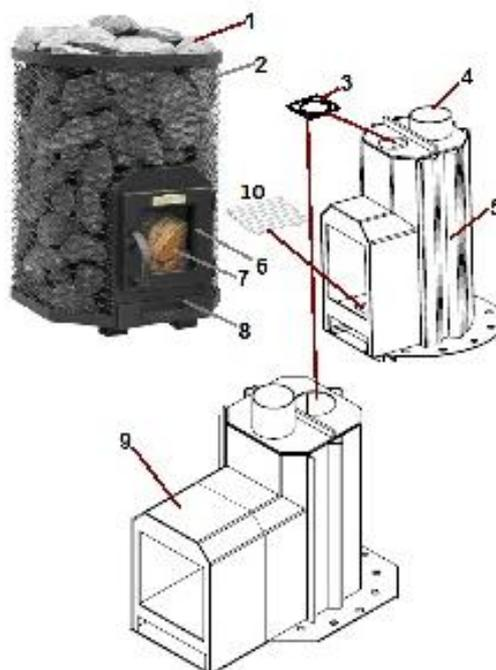
Figure 1. Heater components
