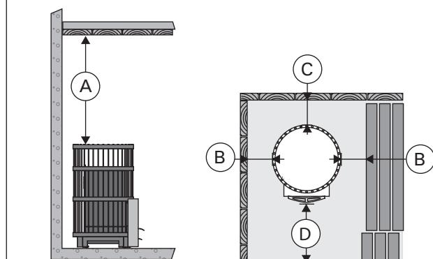
Figure 9. Safety distances (all dimensions in millimeters)
