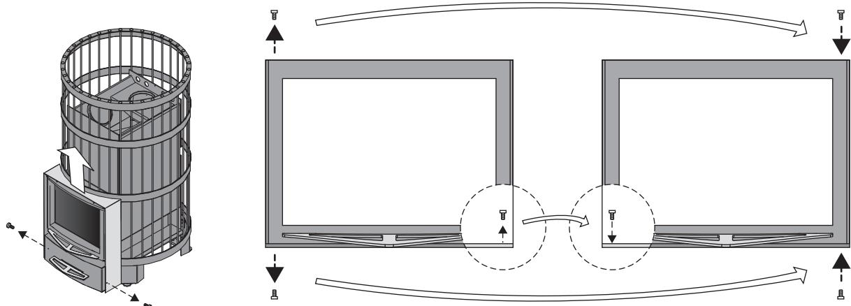
*Figure 15. Changing the opening direction of the stove door
