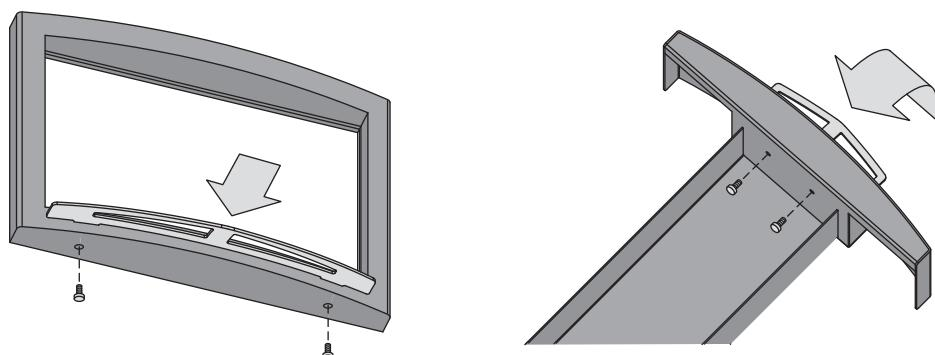
*Figure 16. Installing the handles
