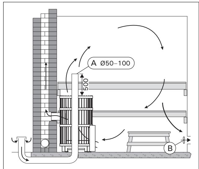
Figure 7. Mechanical exhaust ventilation
