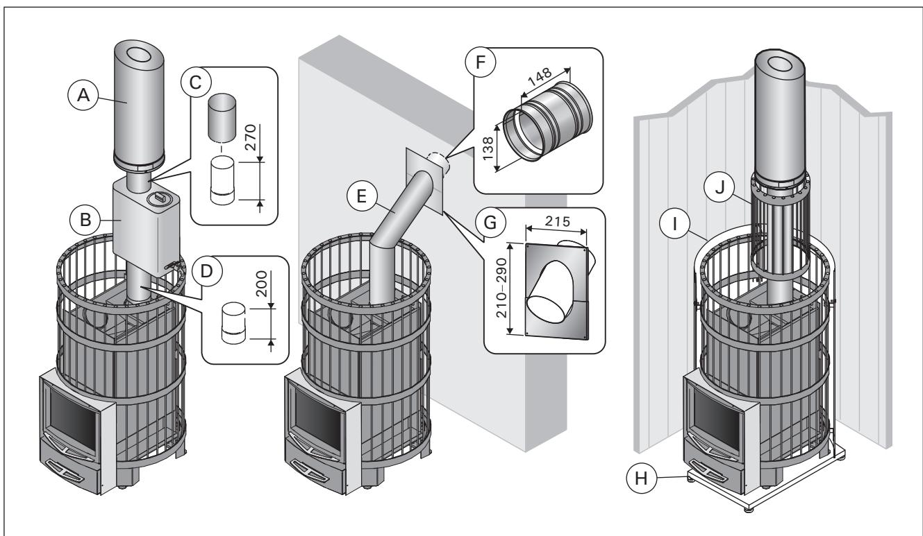
**Figure 17. Accessories (all dimensions in millimeters)**
