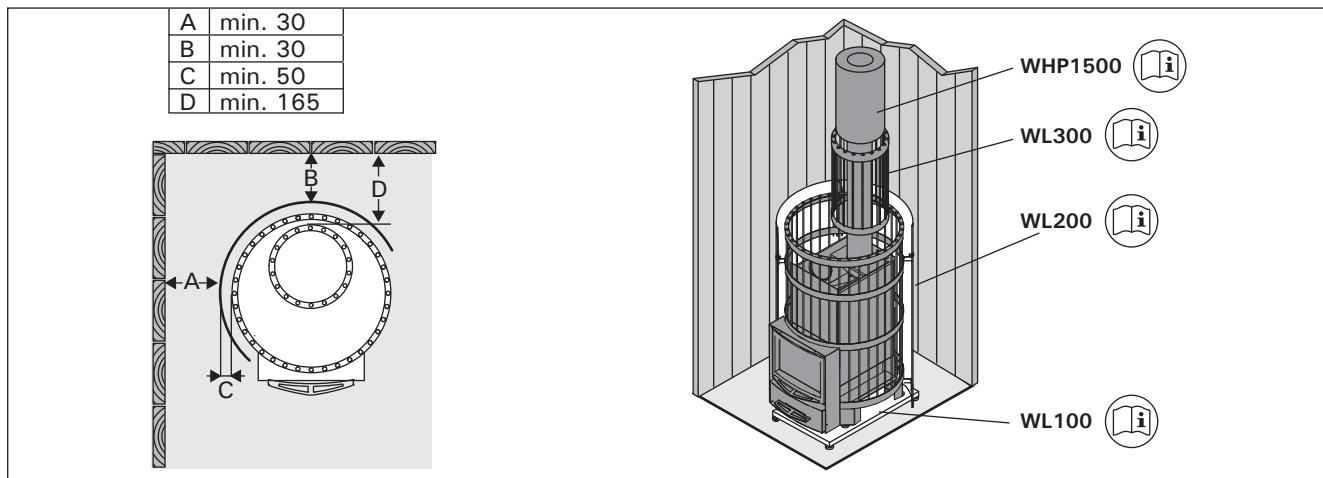
Figure 10. Legend Protection Supplies (all dimensions in millimeters)
