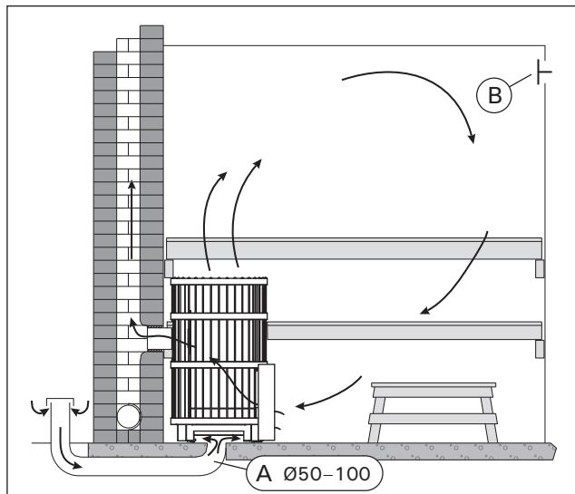
Figure 6. Gravity exhaust ventilation
