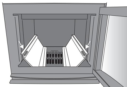
**Figure 2. Combustion air channels**
